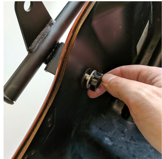
figure 3. attaching saddlebags to bracket
